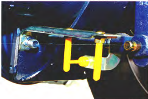
TRAILER AXLE - BRAKE RELEASED POSITION
